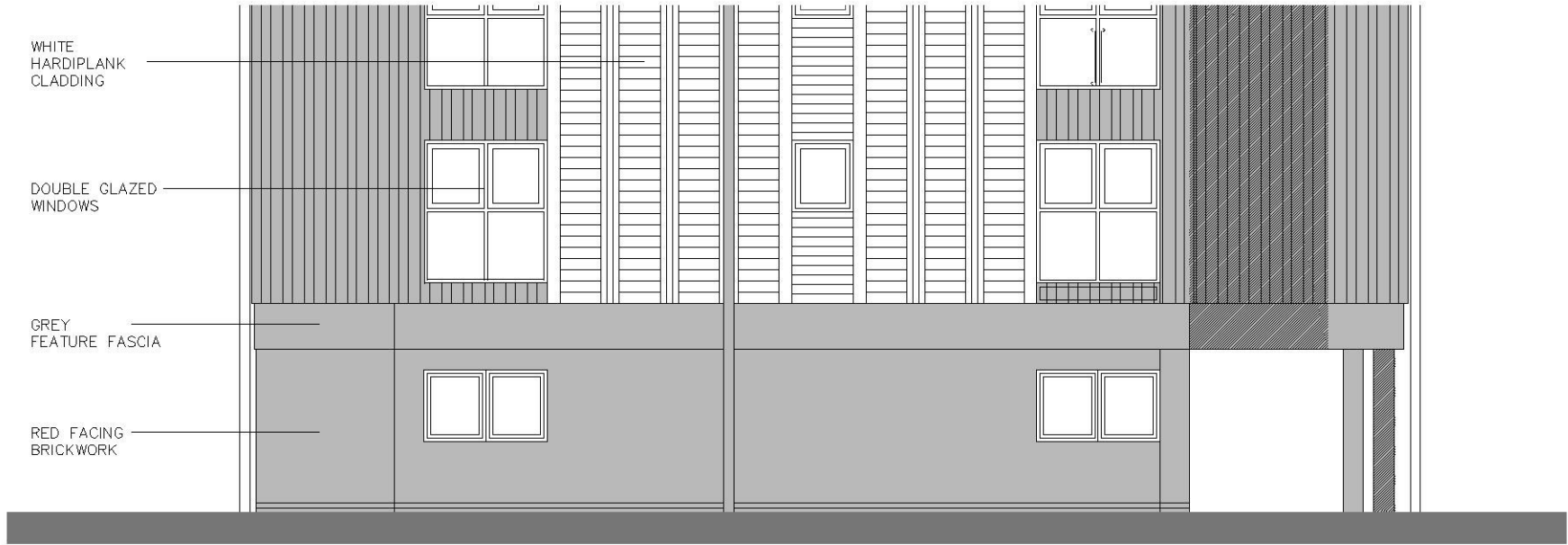
South West Elevation @1:100
