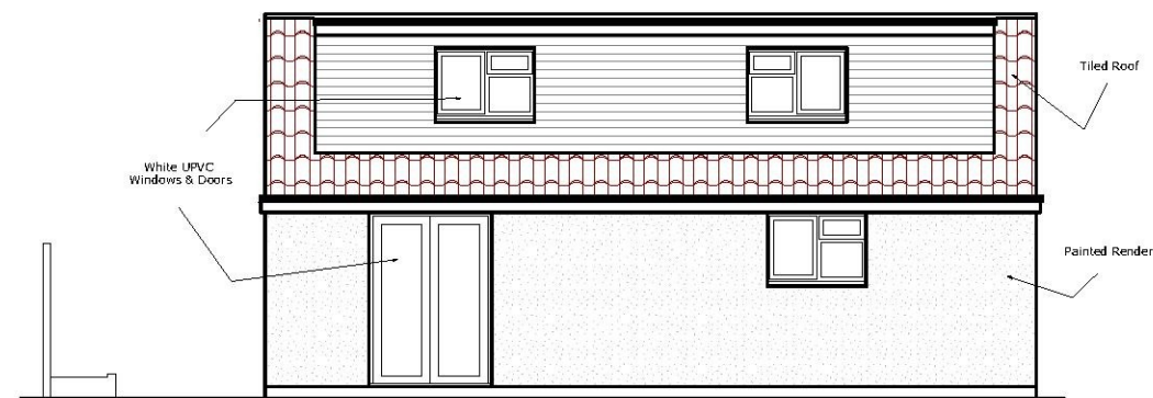
Existing Rear Elevation
