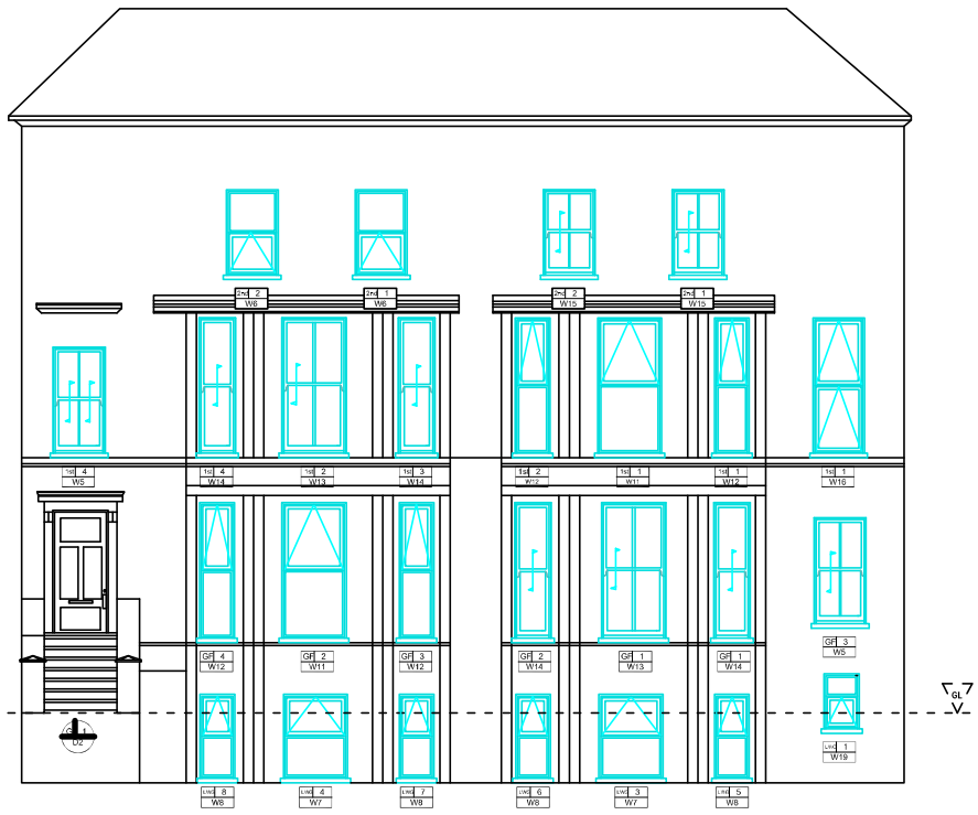
Existing no. 58 Front Elevation
