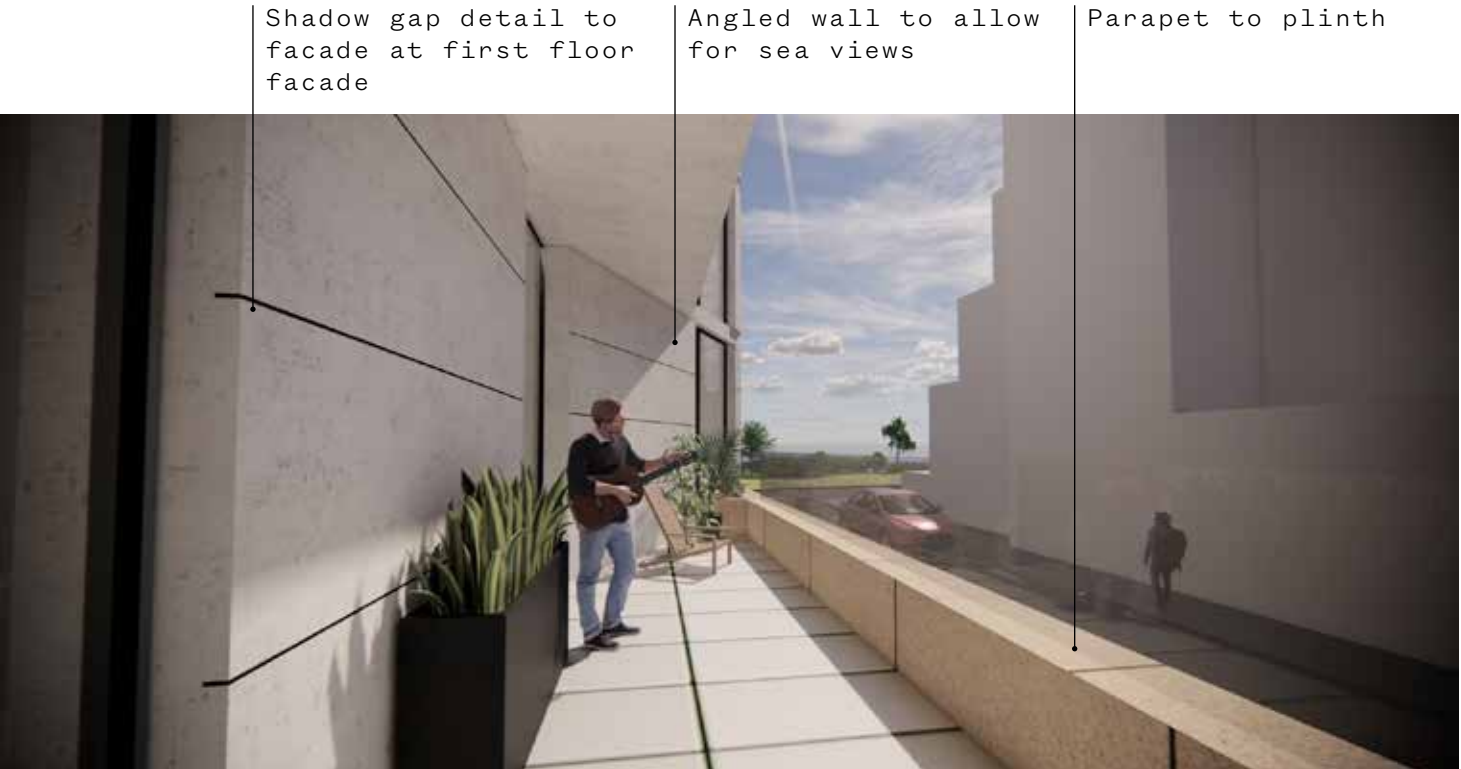
Plinth and balcony to Cheriton Place
