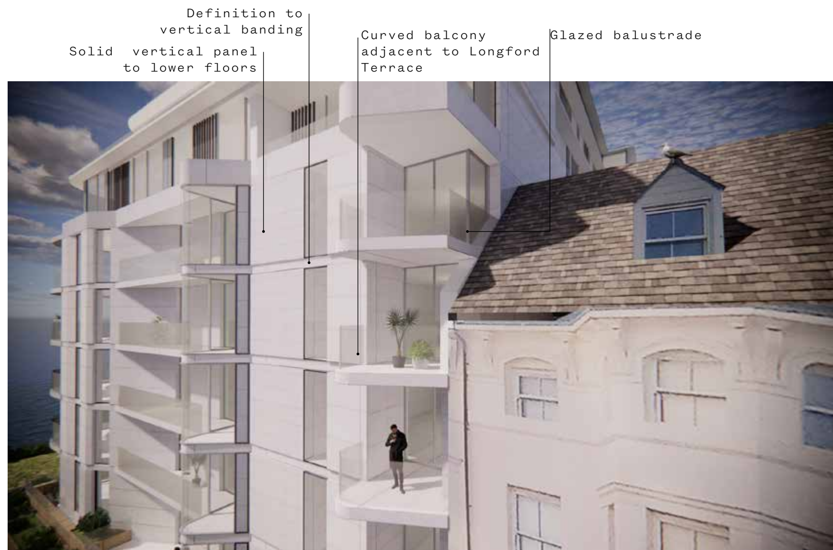
Proposed Building adjacent to Longford Terrace
