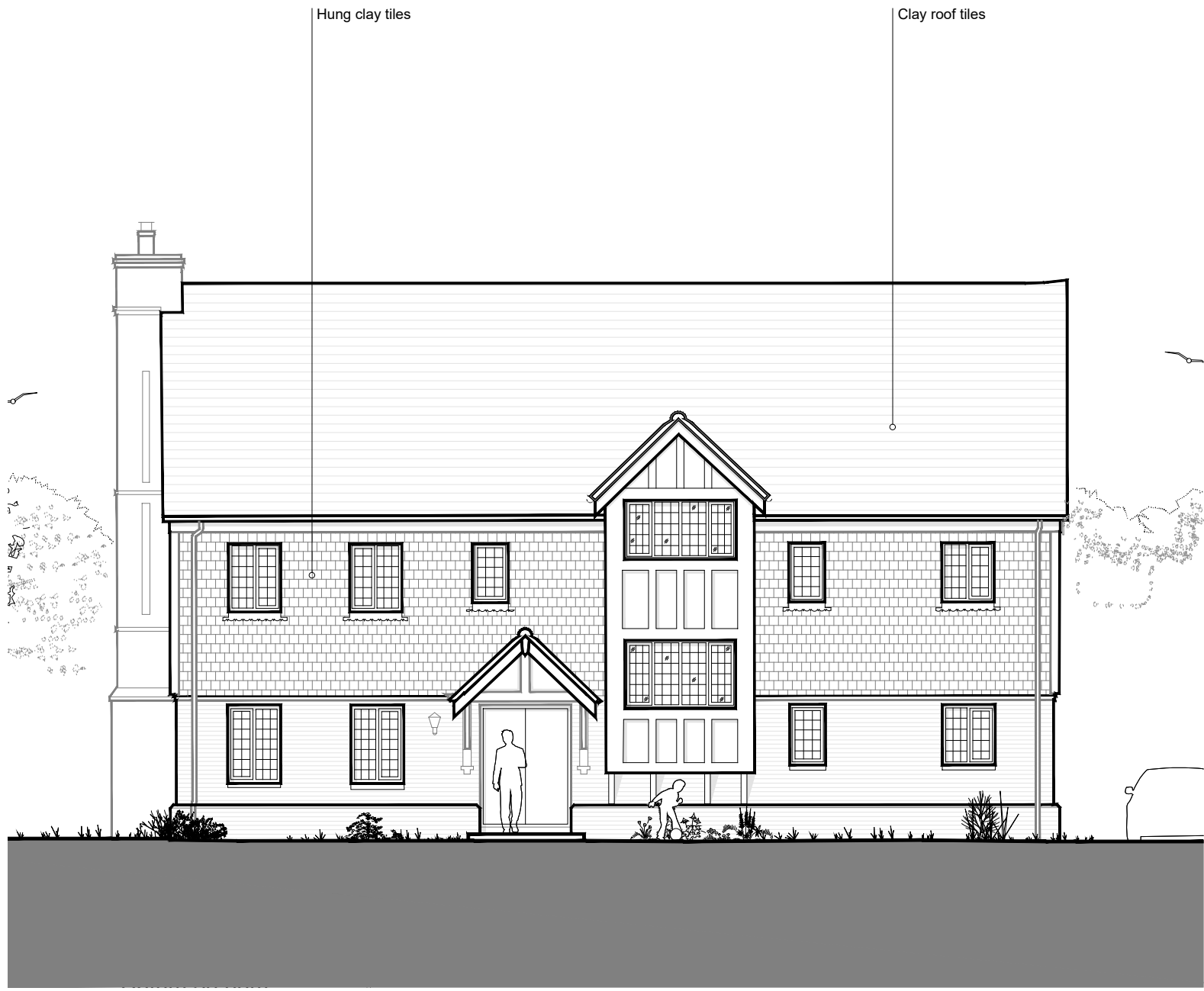
EXISTING NORTH ELEVATION 1:100 @ A1
