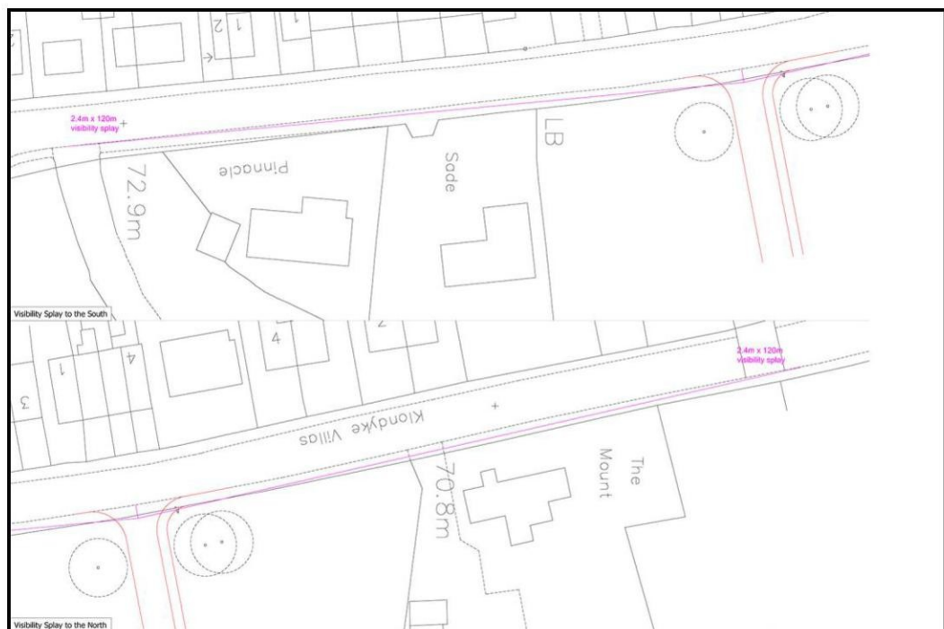
Figure 14. Visibility splays at the access.
