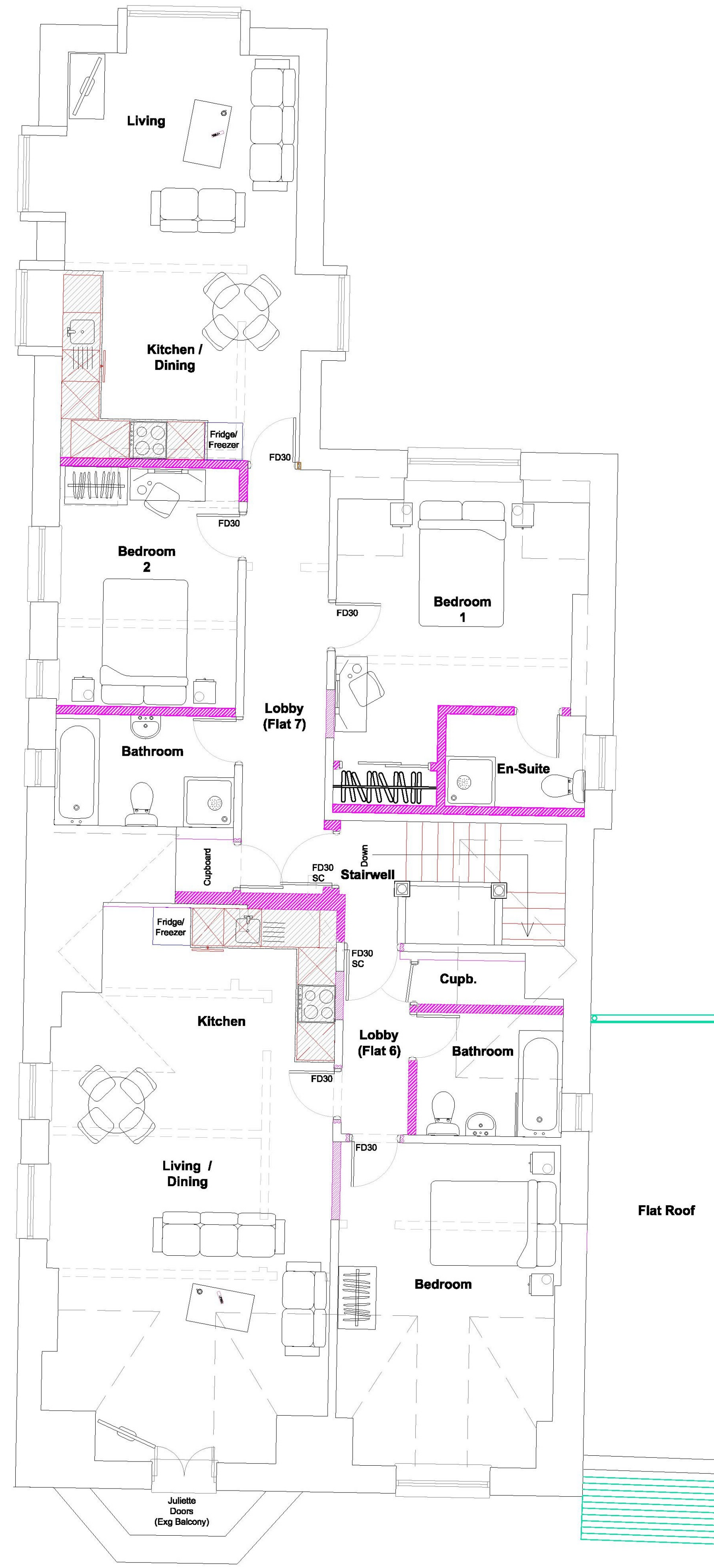
Proposed Second Floor - Two Self Contained Flats No. 76 (1 No. 2 Bedroom & 1 No. 1 Bedroom Flat) Scale 1:50
