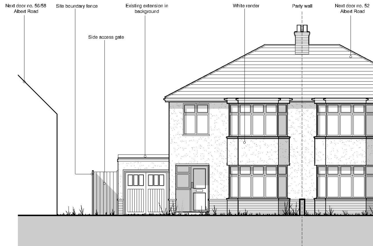
EXISTING FRONT ELEVATION
