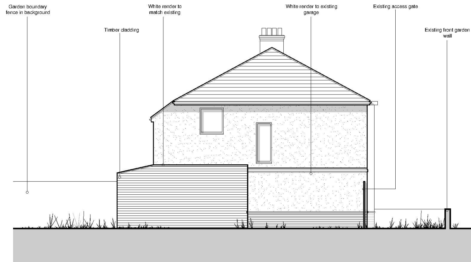
EXISTING SIDE ELEVATION
