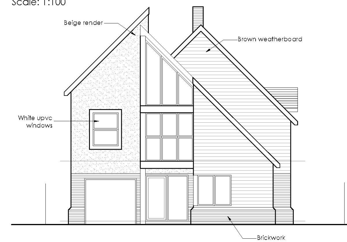
South West Elevation
