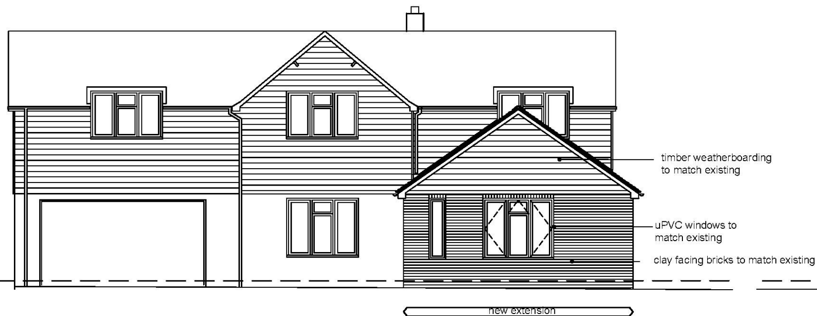
NORTH WEST ELEVATION
