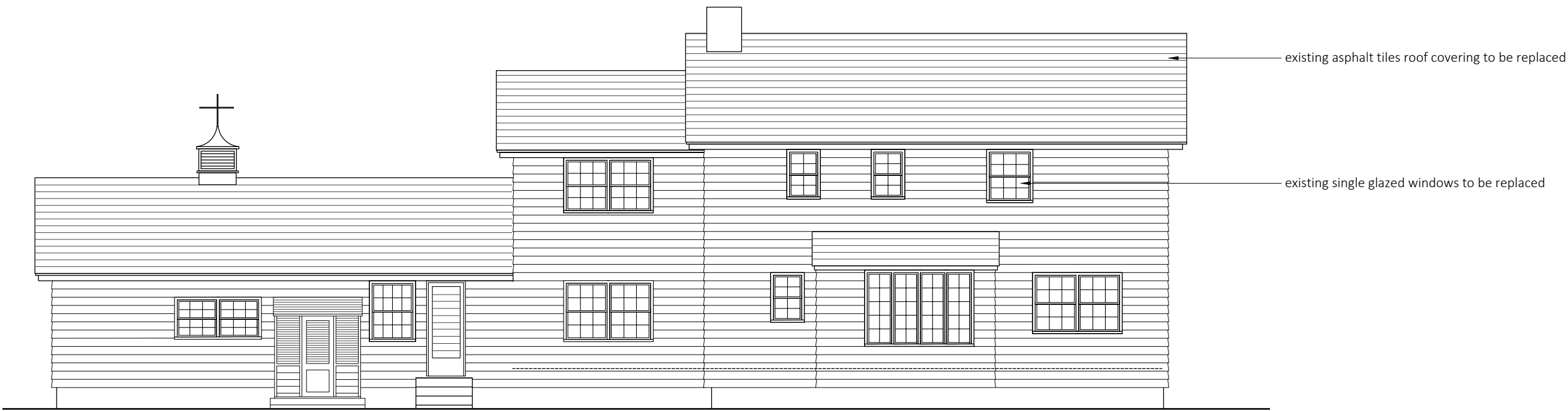
existing east (rear) elevation 1:100
