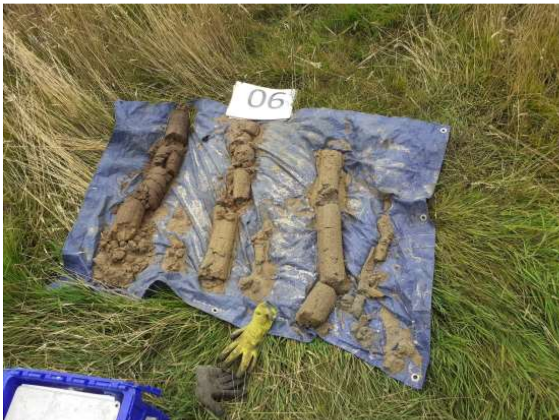
Image of the 1 st to 3 rd metre (left to right) of sample retrieved from BH06
