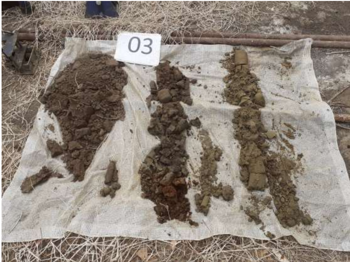
Image of the 1 st to 3 rd metre (left to right) of sample retrieved from BH03
