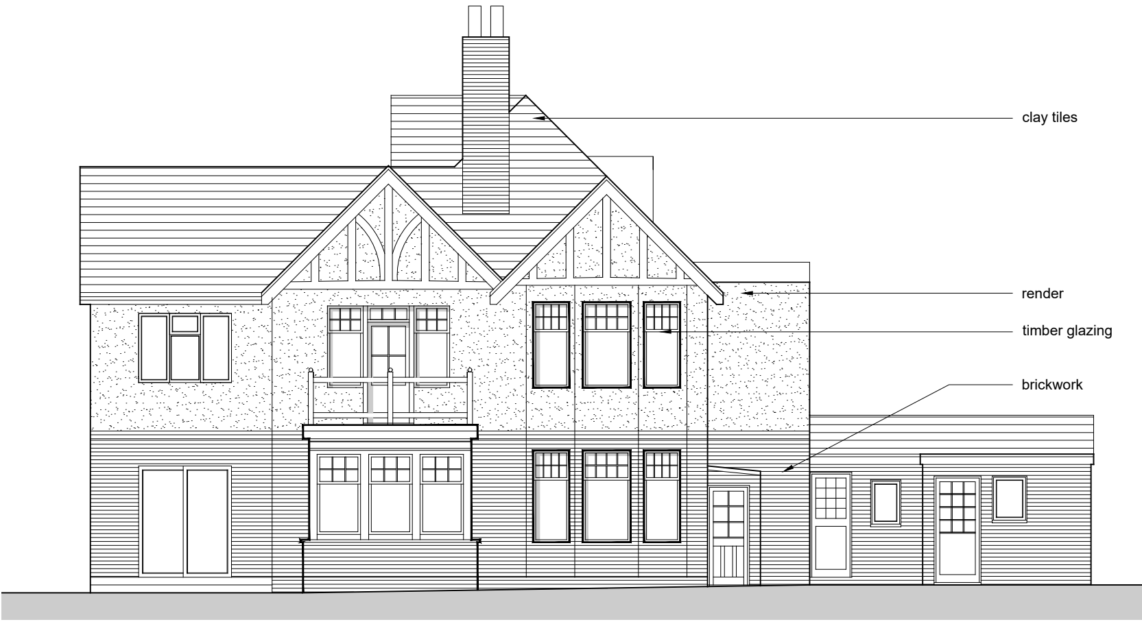
Existing South Elevation
