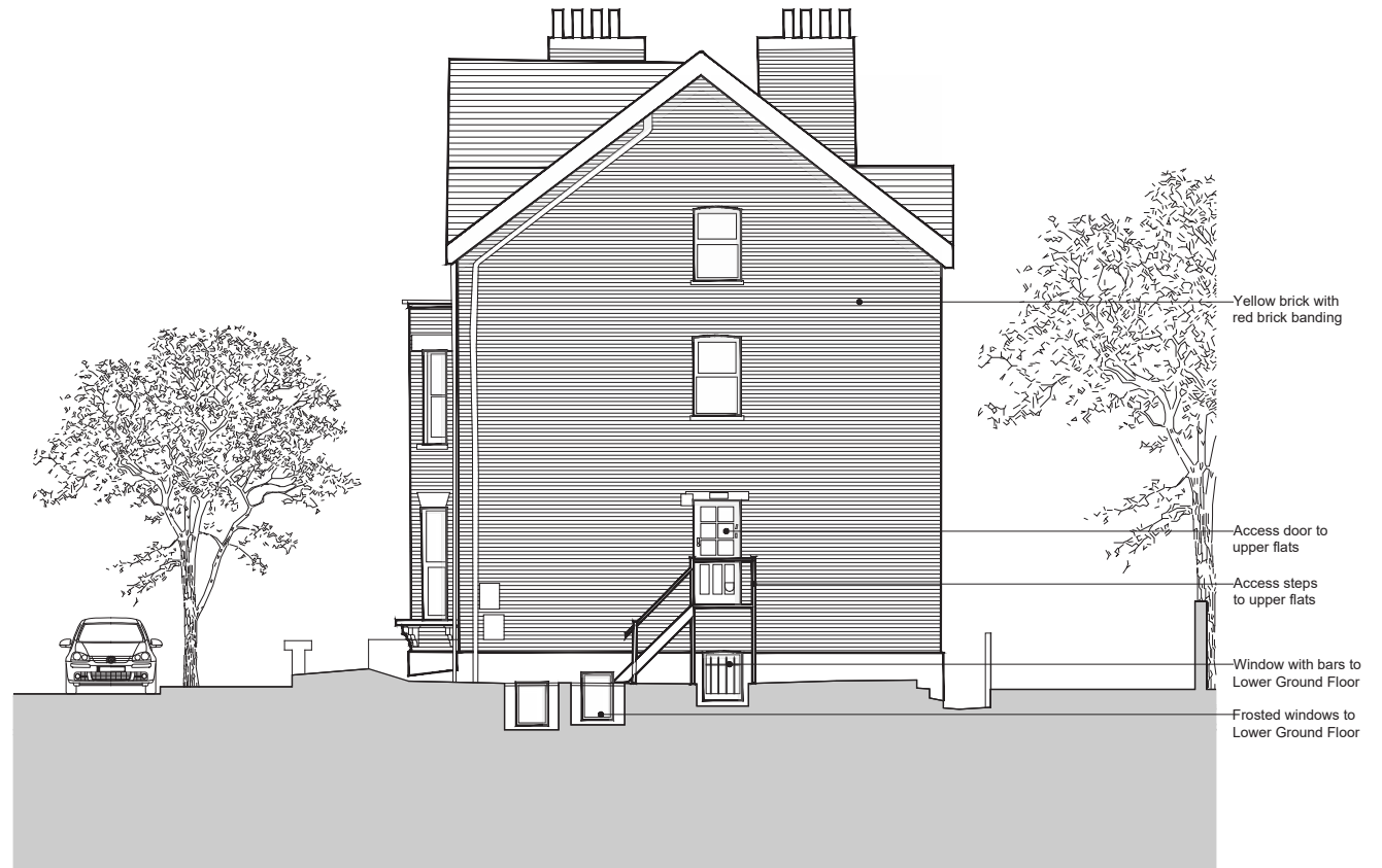
Existing West Elevation
