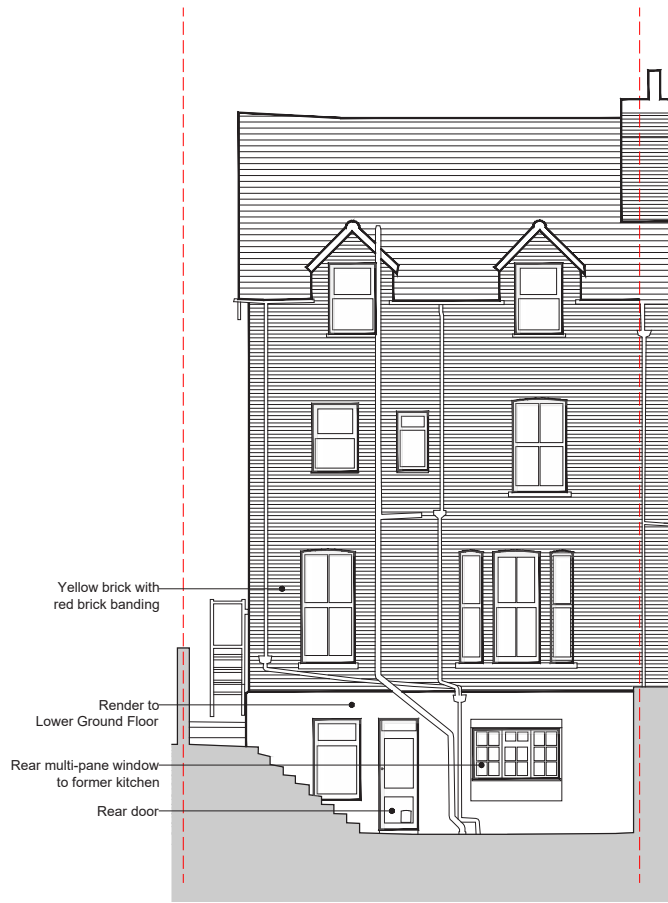
Existing South Elevation
