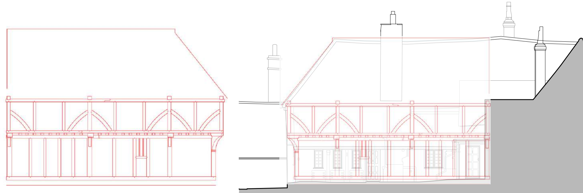
CANTERBURY ARCHAEOLOGICAL TRUST - Partial reconstruction showing suggested medieval arrangement of east wall
