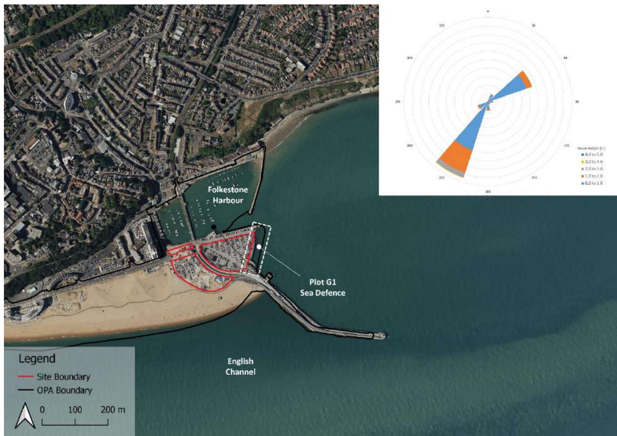
Figure 5-2 Location of Plot G1 Sea Defence with a wave rose showing the significant wave height for the UK MetOffice hindcast point offshore (extracted from Folkestone Seafront Harbour Masterplan Development – Coastal/ Wave Modelling Report (document no. PC4284-RHD-XX-ZZ-RP-0103-S3-P01-2) (RHDHV, 12/05/2023))
