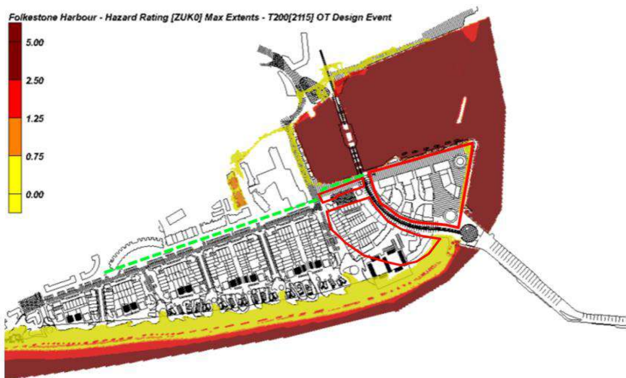
Figure 8-2 Safe access and egress from Plot E1 (red line boundary) to areas outside maximum flood extent. Evacuation route identified in Green. Hazard Rating: <0.75 – very low hazard, 1.25 – Danger for some, 2.5 – Danger for Most, >2.5 – Danger for all
