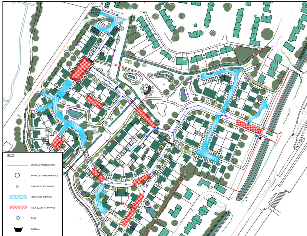
Figure 8.1 - Indicative drainage layout plan showing the proposed location of SuDS.
