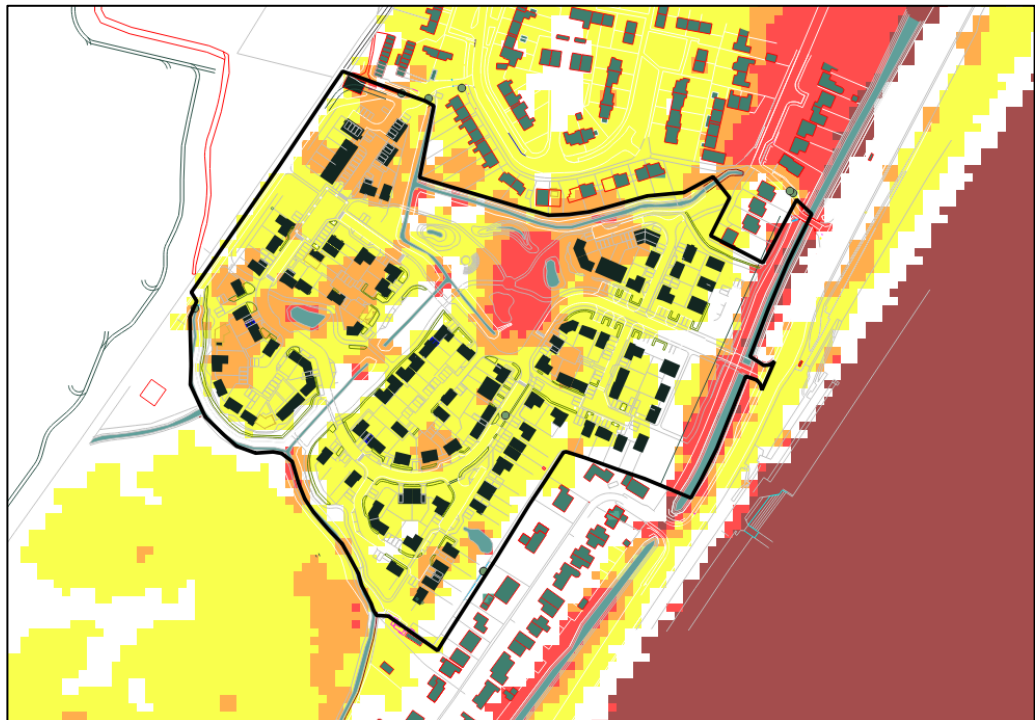
Figure 6.1 – Hazard rating classification on site during a breach at Hythe Ranges under design conditions. Site boundary delineated in black. See Table 6.1 for key.
