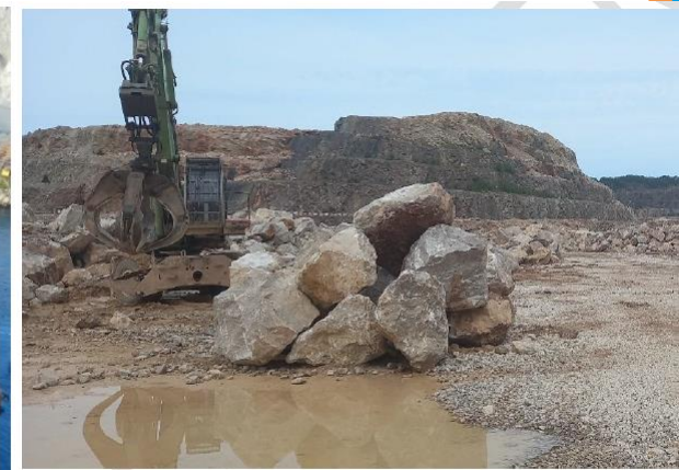
Figure 2: Quarry floor in Bolougne, showing sorting of 3-6t rock grade
