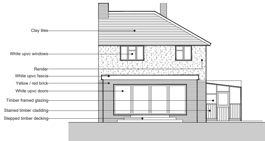
Existing Rear Elevation (South)
